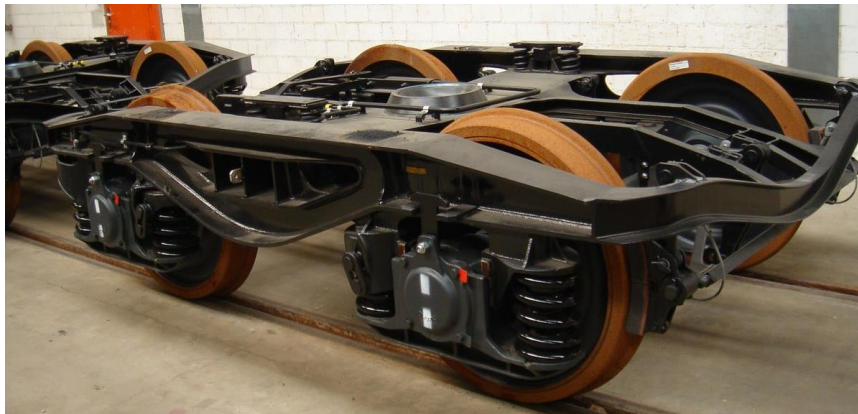
Fig. 22: Y25 freight wagon bogie [45]
